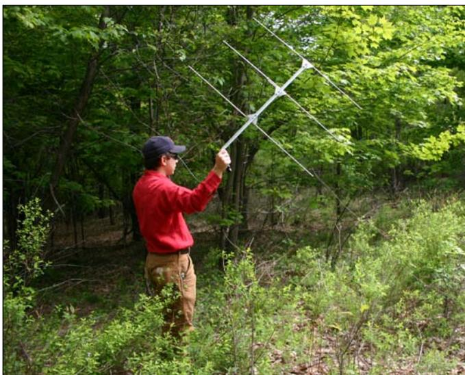
**Figure 14. Taking radio telemetry locations with a 3-element yagi antenna.**
