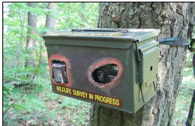
**Figure 50. A modified ammunition box housing a remote camera used to record images of bears visiting a taste aversion bait station in 2005.**
