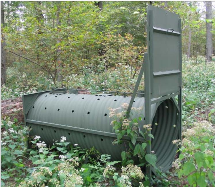
**Figure 6. Side view of “Fort Drum hybrid” culvert trap.**
